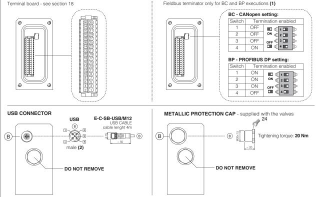
(1) Drivers with BC and BP fieldbus interface are delivered by default 'Not Terminated'. All switches are set OFF (2) Pin layout always referred to driver's view
